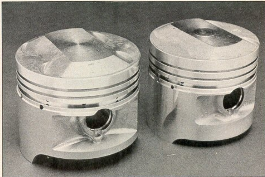
Yoshima's 68mm, 11.3:1 piston (left) boosts displacement to 1002cc. A stock 62mm CB750F piston is shown at right.
